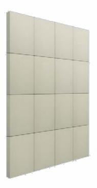
Blasblock Acoustic, SoundAbsorber has been tested in accordance with ISO 354 Acoustic Measurement of sound absorption in a reverberation room and exhibits Noise Reduction Coefficient (NRC) of 0.55 which typically reduce reverberated noise by approximately 55%
